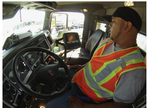
Nalco Champion's trucks were equipped with a Motorola VC6090, a truck mounted mobile computer, and Option Technologies Corp. CloudGate modems, allowing trucks to connect with any cellular network. Satellite modems were also installed in some trucks, allowing for constant communication with the vehicle concerning service work and driver safety.
